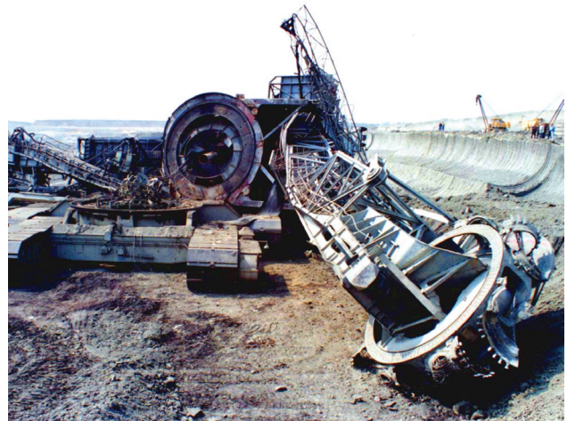
Figure 5 – Look of bucket-wheel excavator SRs 1200 24/4 (G2), after the accident which occurred on April the 6th 1995.
