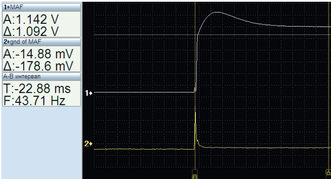
Figure 2. An output voltage oscillogram of a sensor from an automobile that had travelled 60 ths km.
