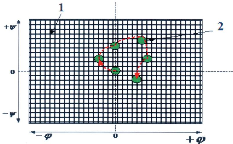
Fig. 2. Evolution of a light emitting diode image on a pixel field of a CCD matrix: 1 – pixel field of a CCD matrix; 2 – image
