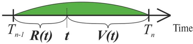
Fig. 1. Modeling of failure points for calculation of residual time
