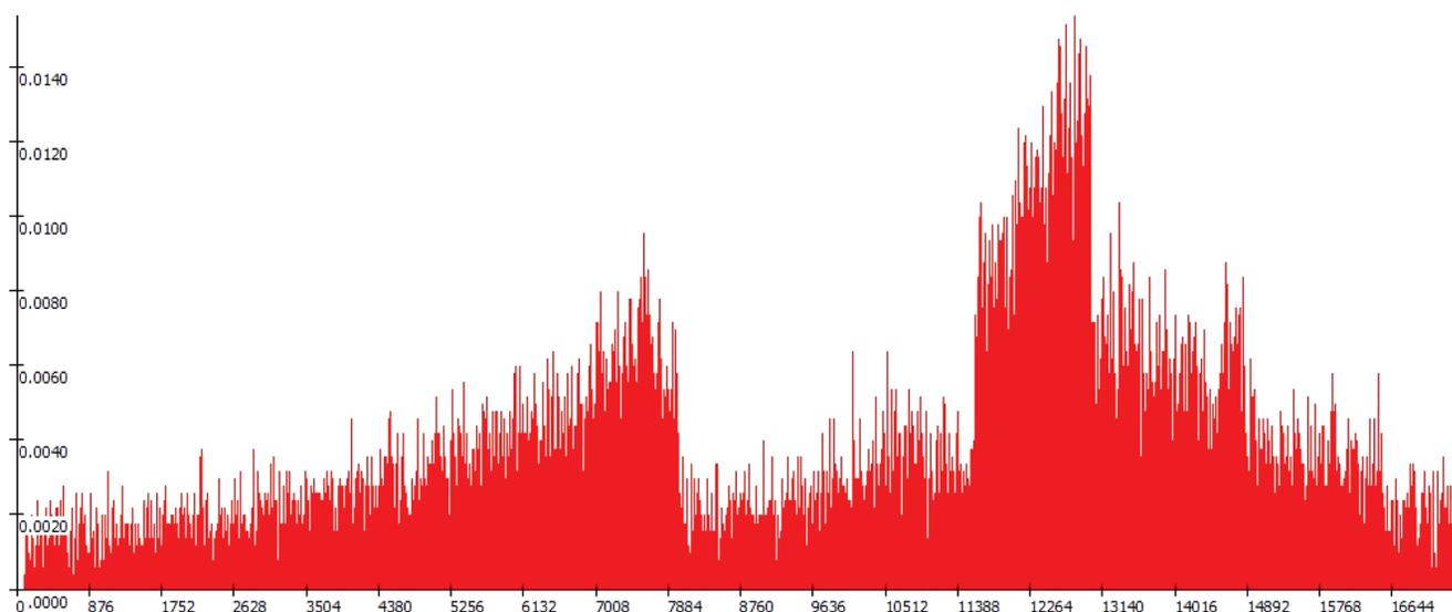
Fig. 5. The diagram of failure frequency of the whole air-conditioning system ADS in time after the changes to the maintenance plan
