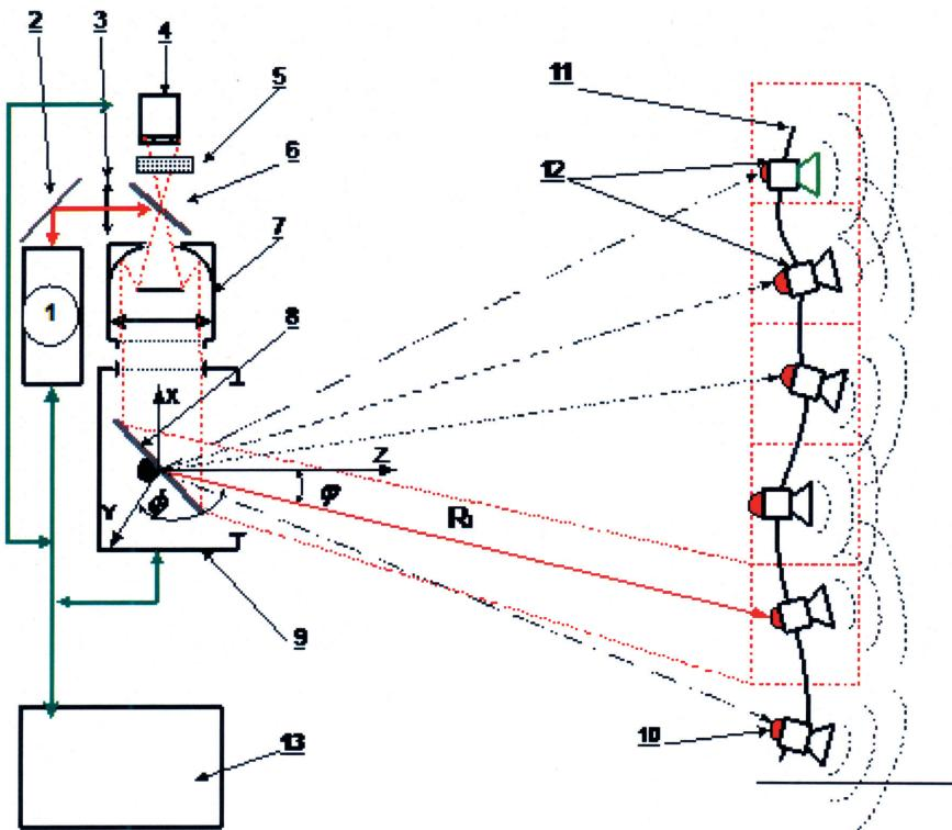
Fig. 1. Model of the device for control of coordinates of PA elements: 1 – laser ranger, 2 – rotary mirror, 3 – focusing lens, 4 – CCD matrix, 5 – light filter, 6 – partially reflecting mirror, 7 – long-focus lens, 8 – moving mirror, 9 – optical scanner, 10 – reflecting elements, 11 – basic structure, 12 – receive/transmit modules, 13 – controller
