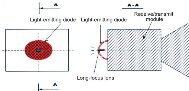
Fig. 3. Structure of a reflecting element and a light emitting diode of the lightning
