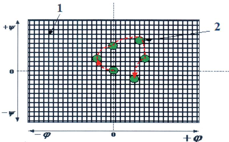
Fig. 2. Evolution of a light emitting diode image on a pixel field of a CCD matrix: 1 – pixel field of a CCD matrix; 2 – image
