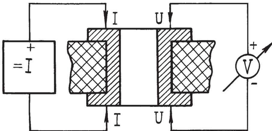
Fig. 9. Scheme of measuring the resistance of hole metallization by four-probe method
