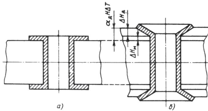
Fig. 2. Distortion of metalized holes when heated
