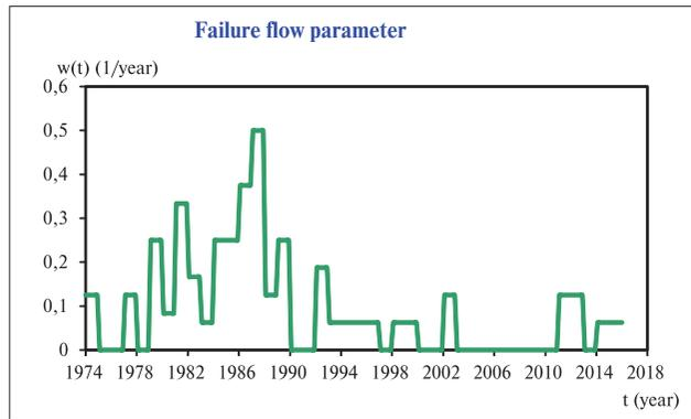
Figure 2. KNK-56 failure flow parameter
